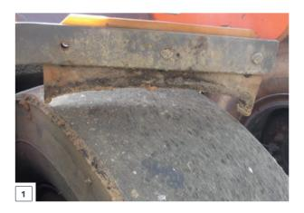
When the surfaces of the drums and tyres are no longer reliably cleaned, worn scrapers should be replaced.
