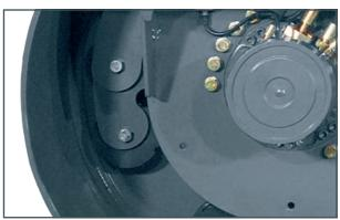
Due to the optimal hardness grade, the compaction energy can be optimally transmitted into the substrate. Incorrectly dimensioned rubber buffers can severely reduce compaction performance.
