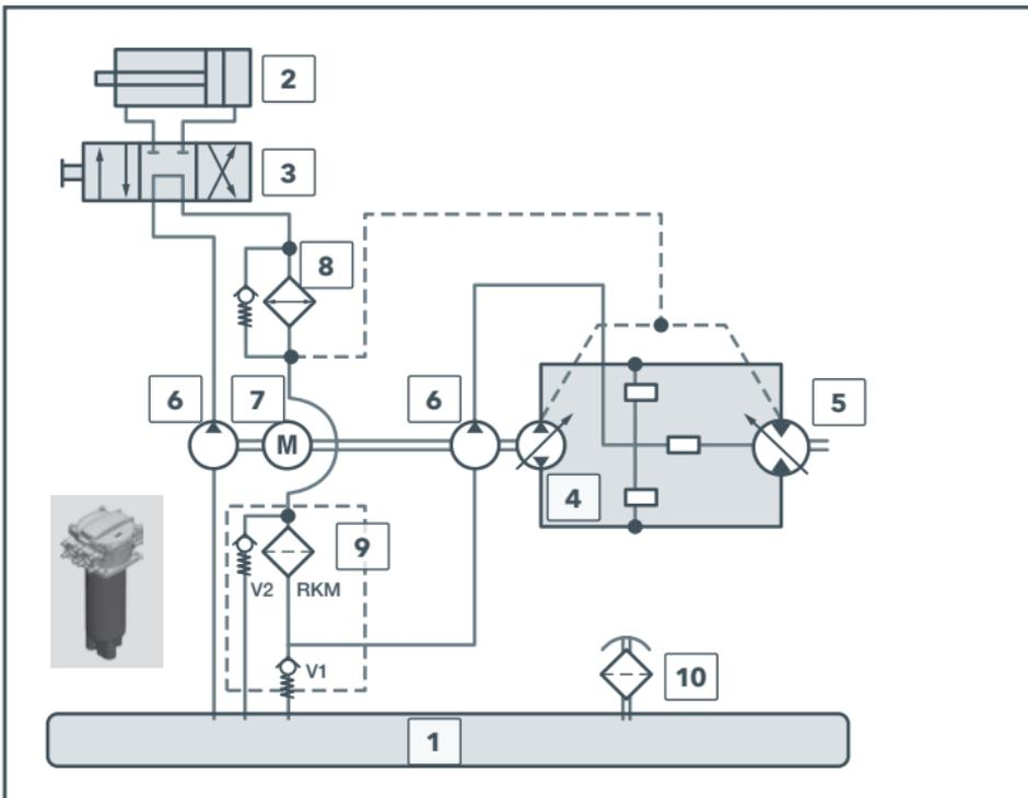
If the leak oil from the hydrostatic drive is routed through the filter in addition to the quantity from the open circuit, care must be taken that the permissible leak oil pressure at the filter is not exceeded in order to protect the radial shaft sealing rings (taking the pressure loss of the leak oil pipes, oil cooler and pressure relief valve into consideration).
