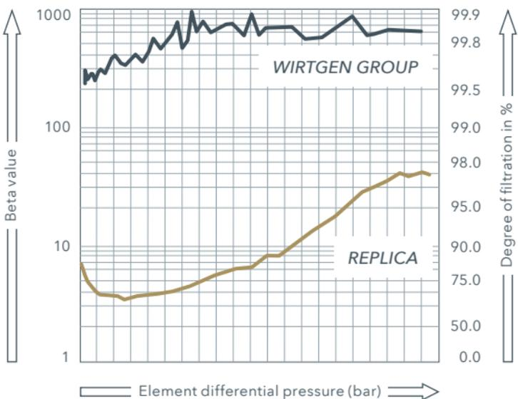
> Seen on the example of a WIRTGEN GROUP hydraulic filter of the same type
