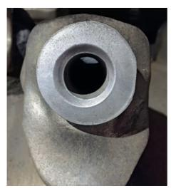
> HT22 quick-change toolholder system after a service period of at least 50 operating hours with a W6/20X pick.
